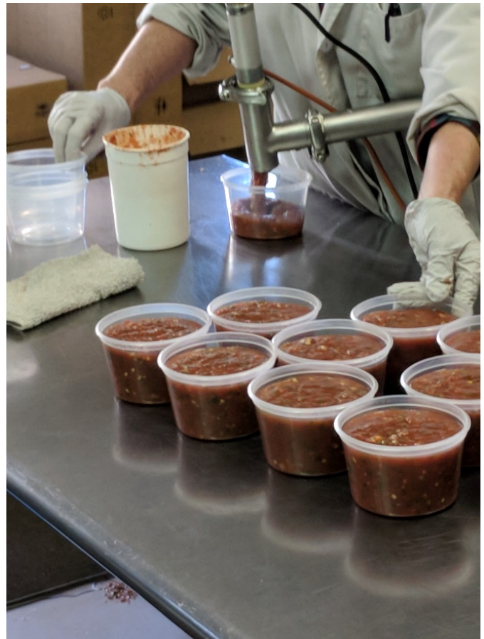
Salsa being co-packed into plastic containers using an extruder to meter the correct amount.
